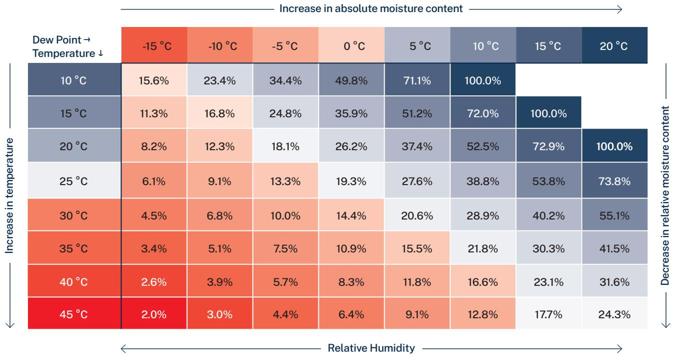
Relationship between Dew Point temperature, Relative Humidity and air temperature. With a Dew Point of 20°C, Relative Humidity can range from 100% right down to 24.3% depending on the air temperature. A general rule is the further apart the air temperature is from the Dew Point temperature, the lower the Relative Humidity of the air above the fire ground.
