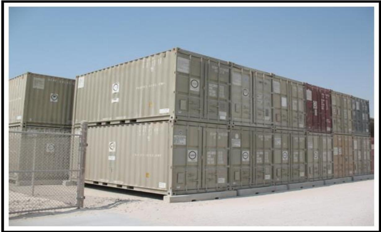
Figure 9: Storage configuration all doors accessible to firefighters
